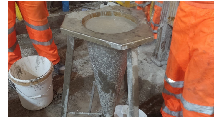
O-funnel testing and measuring concrete flow
